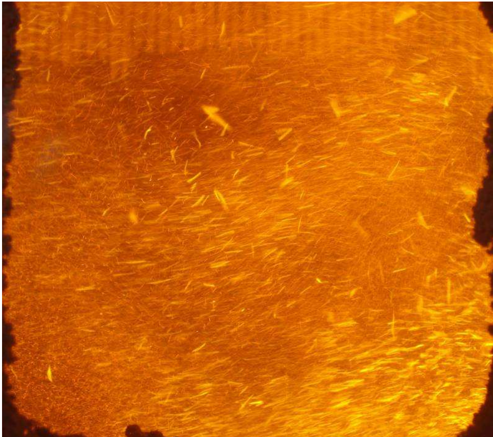
Fig. 15 – TEA-C EFS burner in PKS firing at 6 t/h biomass feeding rate
