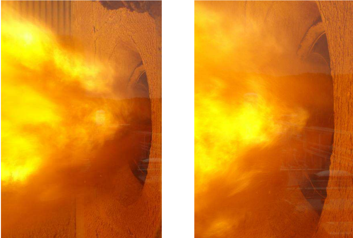
Fig. 14 – TEA-C EFS burner in full WP firing at 6.5 and 7 t/h biomass feeding rate
